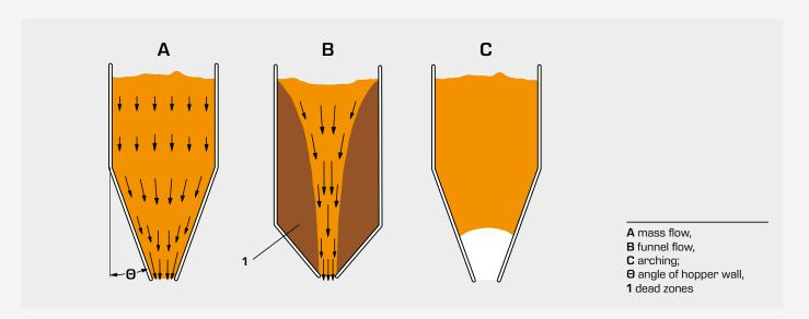
Whether mass or funnel flow is occurring depends on the flow properties of the bulk solid and on the wall material and angle of inclination of the hopper walls. The required angle of the hopper walls can be calculated if the flow properties are known. The
