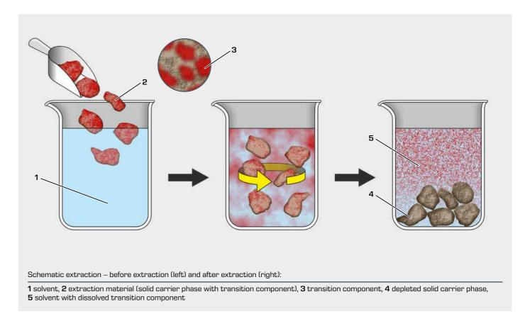
To achieve the fastest and most complete solid extraction possible, the solvent must be provided with large exchange surfaces and short diffusion paths. This can be done by pulverising the solid to be extracted. However, an excessively small grain size can cause agglutination and make it more difficult for the solvent to permeate.
