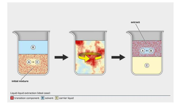
The example illustration assumes an ideal situation in which the transition component A is completely taken up by the solvent. In reality, residual transition component always remains in the carrier liquid. In addition, complete insolubility of the carrier liquid in the solvent is assumed. In practice, parts of one substance will always be found in the other.
