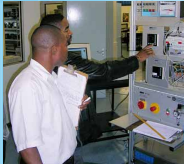
Operation and parameterisation of a digital controller via keypad
