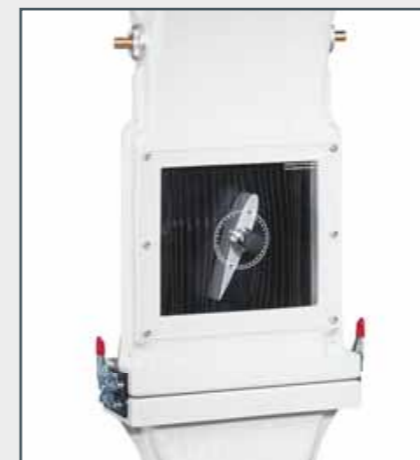
Separation of the flow on the right side by changing the angle of attack
