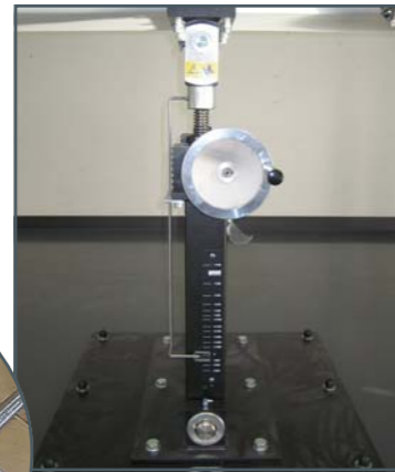
Jacking support for inclination adjustment
