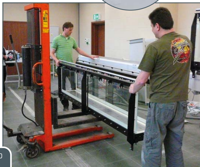
The experimental section element is placed on the carrier with a forklift, aligned and installed.
