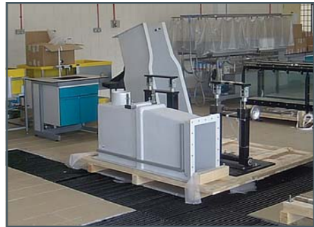
Inlet element, outlet element and flume supports
