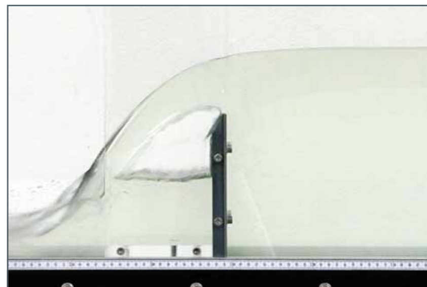
Aerated plate weir (side view)
