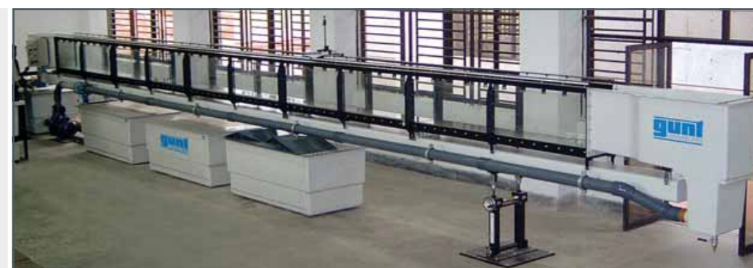
HM 163 with an experimental section of 12,5m
