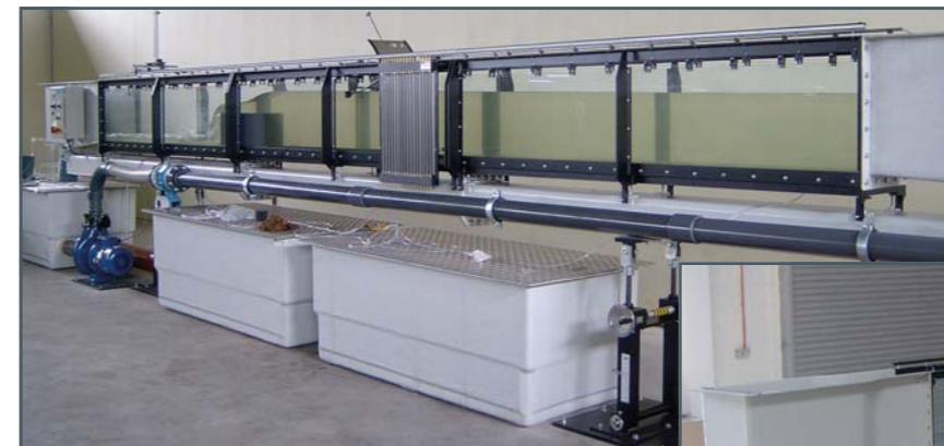
Once installation is complete the system is commissioned; this photo shows the process with the broad-crested weir.
