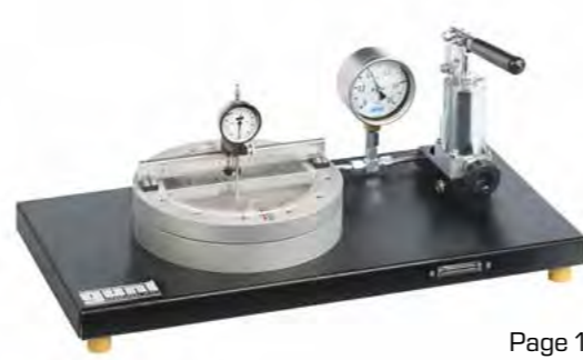
FL 120 Stress and strain analysis on a membrane
