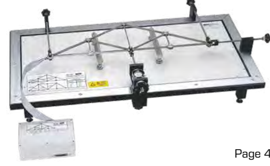
SE 130 Forces in a Howe truss
