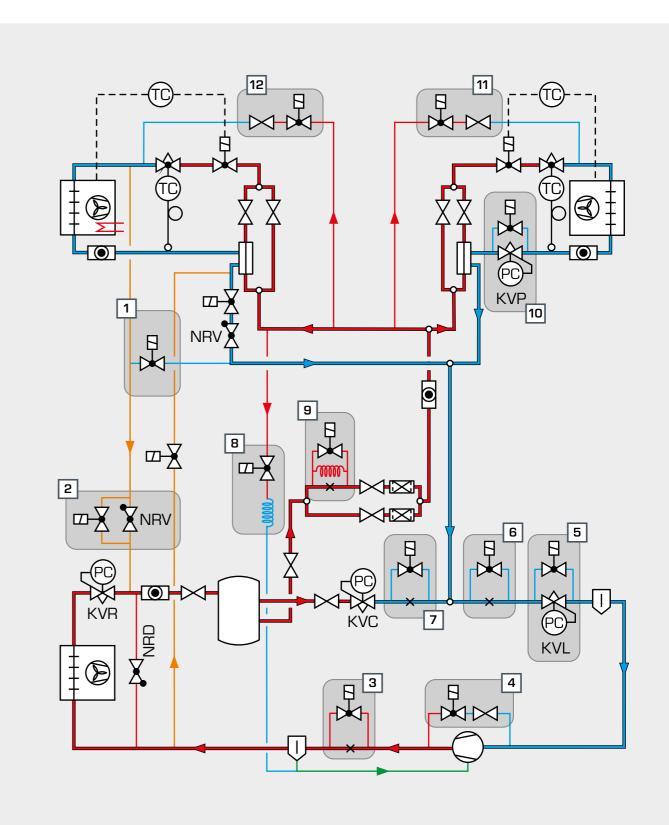
KVP evaporation pressure controller, KVR condensation pressure controller, KVL start-up controller, KVC capacity controller, NRD, NRV non-return valve;
