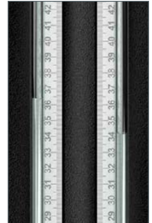
The tube manometer enables low pressure losses to be determined with a high degree of accuracy.
