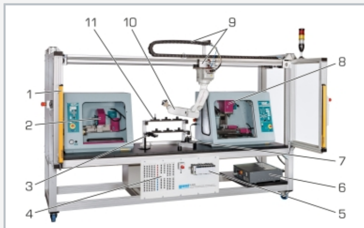
1 safety device (photoelectric barrier), 2 lathe, 3 stock, 4 patchboard, 5 PLC, 6 robot controller, 7 inspection station, 8 milling machine, 9 travel unit, 10 robot, 11 finished parts store
