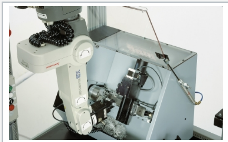
The illustration shows the robot removing a part from the lathe
