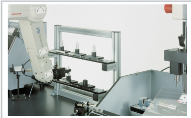
The illustration shows the robot storing a machined part on a pallet in the finished parts store
