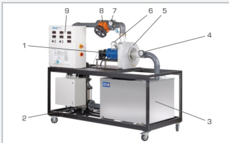
1 asynchronous machine, 2 pump, 3 tank, 4 pressure display at turbine outlet, 5 turbine, 6 adjustment of guide vanes, 7 pressure display at turbine inlet, 8 flow control valve, 9 switch cabinet with displays and controls
