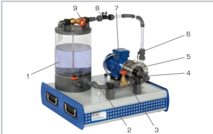
1 water tank, 2 temperature sensor, 3 valve at inlet, 4 pressure sensor at inlet, 5 pump, 6 pressure sensor at outlet, 7 motor, 8 flow meter, 9 valve at outlet
