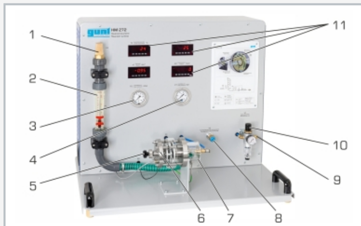
1 silencer, 2 rotameter, 3 outlet manometer, 4 inlet manometer, 5 brake torque adjustment, 6 load unit, 7 reaction turbine, 8 valve for setting the flow rate, 9 compressed air supply, 10 pressure reducing valve with filter, 11 displays
