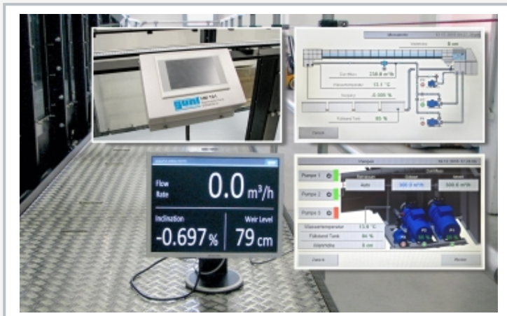
Monitor with display of measured values and operating states, freely positionable touch panel (left) and screenshots of the PLC (right)
