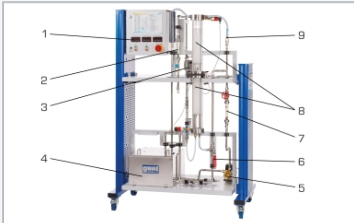
1 digital pressure indicators, 2 air flow meter, 3 compressor for air, 4 storage tank, 5 pump for water, 6 bottom rising-falling switch valve, 7 water flow meter, 8 two-piece packed column, 9 top rising-falling switch valve
