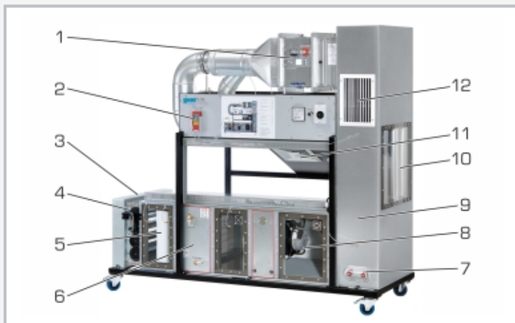
1 fire protection flap, 2 hand-held measuring unit pressure, 3 weather louvre, 4 multi-leaf damper, 5 filter, 6 heat exchanger, 7 inspection cover, 8 ventilator with drive motor, 9 air duct, 10 sound insulation link, 11 ceiling vent, 12 wall vent
