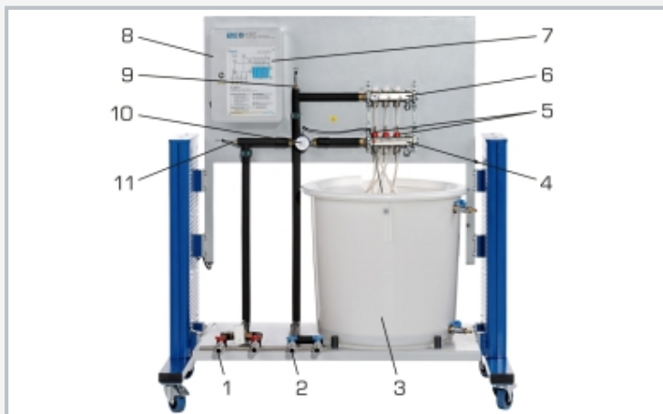
1 connection for feed, 2 connection for return, 3 tanks for hot and cold water, 4 feed distributor, 5 flow meter, 6 return distributor, 7 info panel, 8 connection box for sensors, 9 return temperature sensor, 10 flow meter, 11 return temperature sensor
