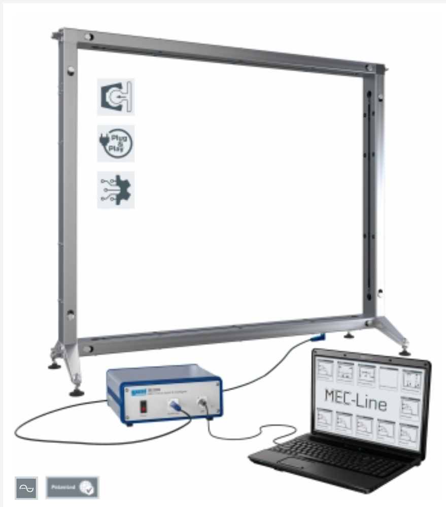
Mounting frame and master module connected via 1 power bus line. Stand-alone capable, optional connection to GUNT software via USB.
