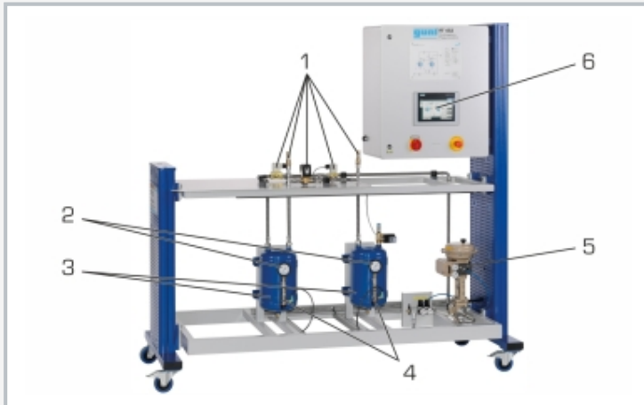
1 various valves, 2 manometer, 3 pressure vessel, 4 smart pressure sensor, 5 control valve, 6 touch screen
