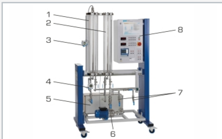
1 tank with two different sensors for level measurement, 2 tank with two free connections, 3 capacitive level sensor, 4 pressure sensor for level measurement, 5 storage tank, 6 pump, 7 external connection option, 8 switch cabinet with connection options
