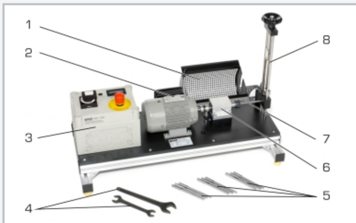
1 protective cover, 2 electric motor, 3 switch box, 4 tool, 5 specimens, 6 bearing, 7 clamped specimen, 8 load application device with spring balance and hand wheel
