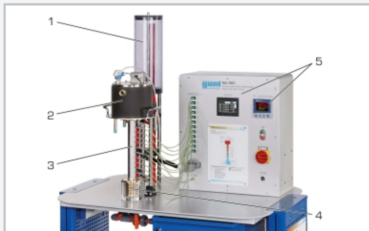
1 elevated tank for constant cooling water initial pressure, 2 heat source with heater, 3 sample, 4 water-cooled heat sink, 5 displays and controls
