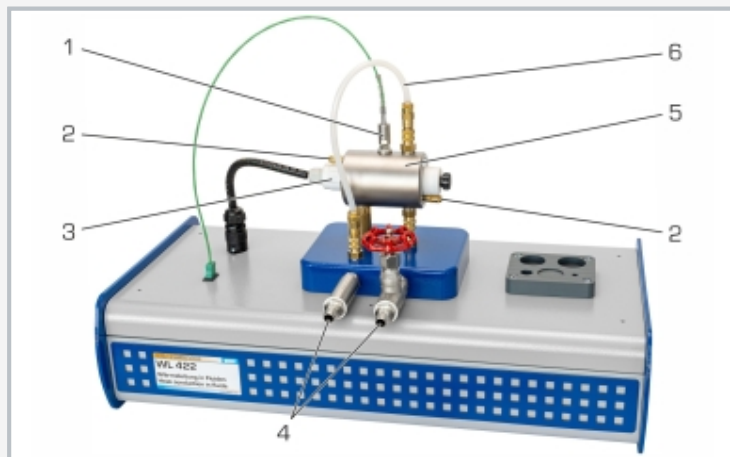
1 temperature sensor, 2 connection for fluid, 3 inner cylinder, 4 valve for cooling water, 5 outer cylinder, 6 cooling water hose
