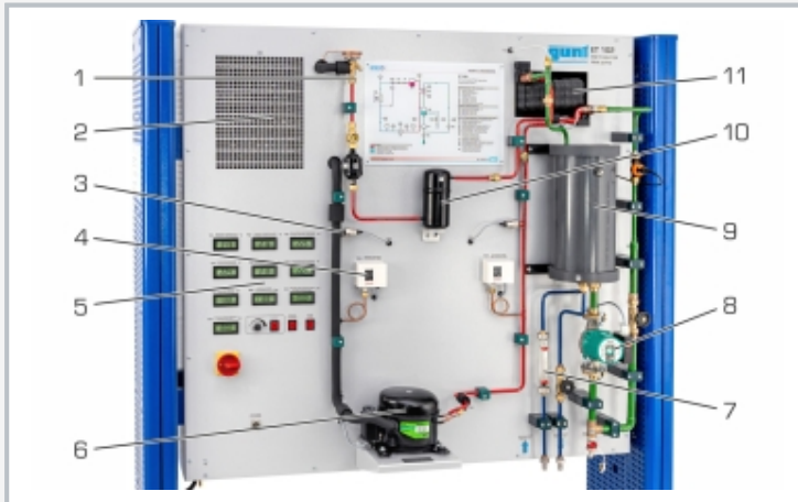
1 expansion valve, 2 evaporator with ventilator, 3 pressure sensor, 4 pressure switch, 5 displays and controls, 6 compressor, 7 cooling water flow meter, 8 pump, 9 hot water tank, 10 receiver, 11 cocondenser
