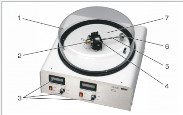
1 protective cover, 2 gyro drive motor, 3 speed displays and adjustment for of the horizontal gyro axis and the vertical precession axis, 4 gyroscopic flywheel mass, 5 lever, 6 sliding weight, 7 inner frame
