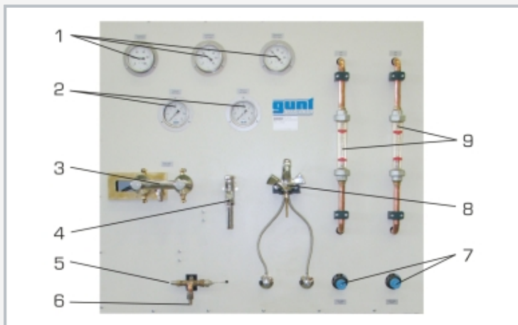
1 thermometer, 2 Bourdon tube pressure gauge, 3 two handle mixer for a shower, 4 flushing valve, 5 mixed water connection, 6 mixed water drain, 7 pressure reducing valve, 8 two handle mixer as water tap, 9 rotameter
