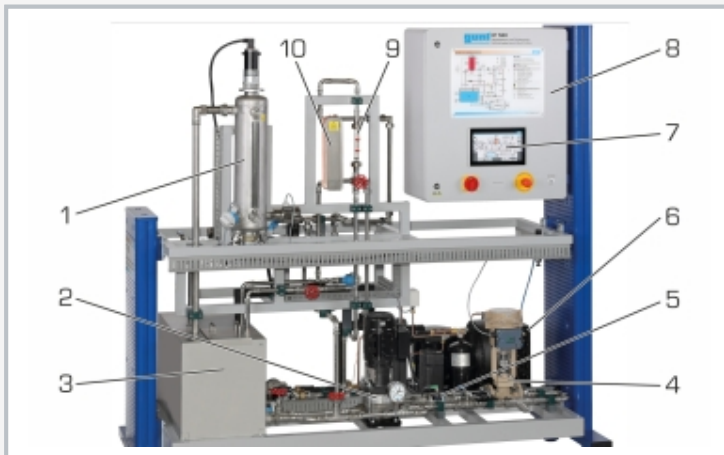
1 stirred tank with heater, 2 main circuit pump, 3 collecting tank, 4 control valve, 5 flow rate sensor, 6 refrigeration system, 7 touch screen, 8 switch cabinet, 9 flow meter, 10 heat exchanger
