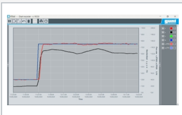
Software screenshot: flow control with PI controller, reference value step
